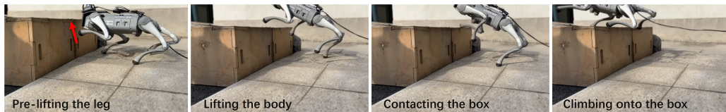
Figure 5: Climbing a wooden box with Lidar
